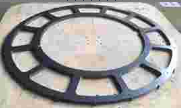
Stamping Laminations for Wind Turbine Generator made by Weser
