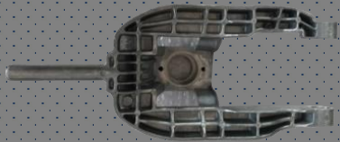
High Pressure Die Cast Auto Shifting Fork Housing for Camaro made by Weser
