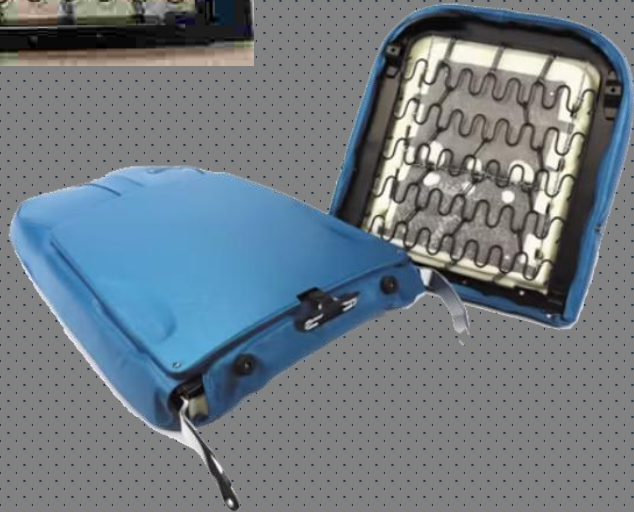
Stamp Seat Back and Bottom Frame for Corvette made by Weser
